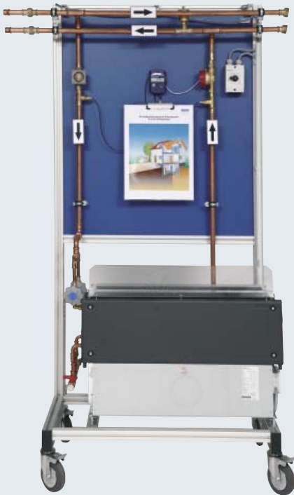
S2 fan convector as the source or the sink
